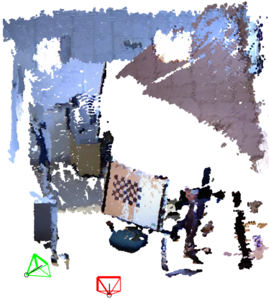
(a) Point cloud obtained with data set A using Kinect 0 and 1 without interference.
